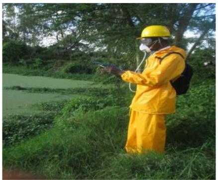
Figure 1. Plate of Karen Brooks settling pond with user taking odour measurements
